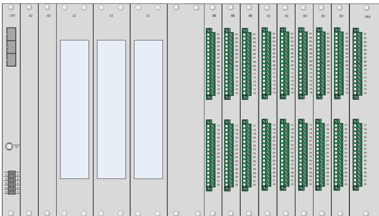
Figure 6.1.5 1/1 19" case rear panel of this relay
